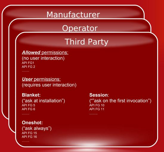
API permission policies for the different protection domains, e.g.3rd party, operator, manufacturer, are dynamically loaded into the device.
