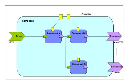
The figure above contains a composite that exposes a RESTful HTTP cloud dashboard service and contains component B1 through Bn, each of which connect to a different cloud provider over a variety of protocols. Component A provides the aggregation, control and presentation necessary for the dashboard service.
