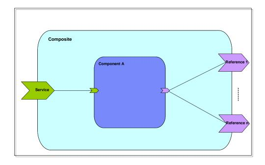
The figure above consists of a single composite that connects to multiple external SIP and PSTN providers. The component also offers a single service that provides the fault-tolerance/load-balancing needed to work around failures, trunk capacity, and policies.
