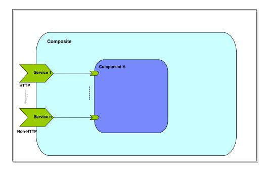
The figure above consists of a composite with a single component that exposes access to the underlying data over multiple protocols/formats by exposing multiple services each with a different binding or format. This provides an ability for the consumer to choose the format/protocol that servers it the best by choosing the appropriate service.
